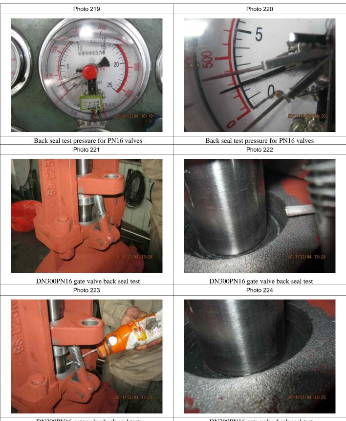
DN300PN16 gate valve back seal test
